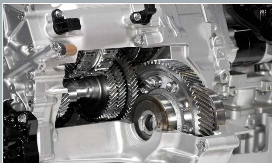
Changing thrust rings in vehicle transmissions from aluminum to high performance PEEK™ provides longer life, lighter weight and easier assembly.
