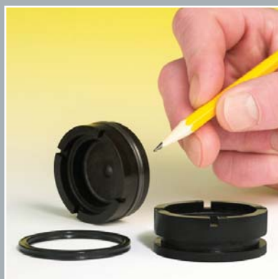
Floating shock absorber pistons changed from aluminum to specially formulated heat-stabilized nylon with Quad-Ring® HNBR seal.
