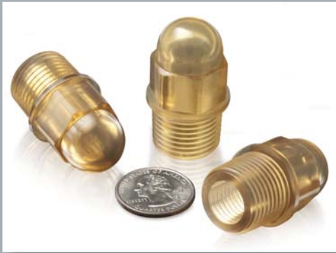
Radiator sight gauge molded as a single component from Polyetherimide (PEI) replaces a more complex three-piece molded and stamped assembly.
